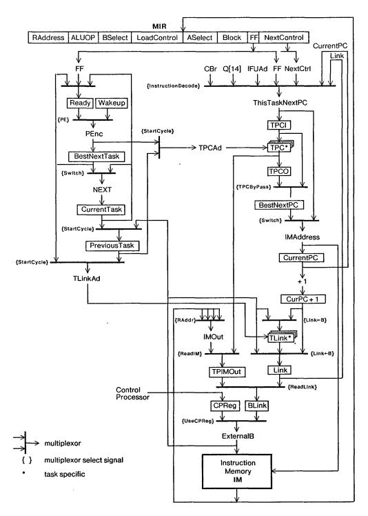
Figure 5: Control section
