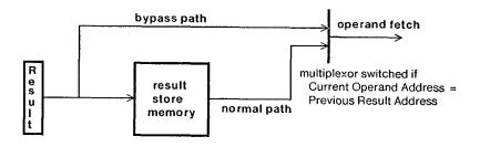
Figure 4: Bypassing example
