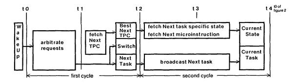
Figure 3: Task arbitration pipeline
