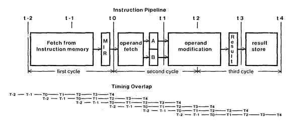
Figure 2: Instruction pipeline and timing overlap
